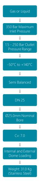
The PRD25 dome loaded pressure reducing valve is both compact and robust in construction making it the ideal solution for a wide range of applications.
